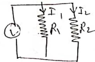
$$V = I_1 R_1 = I_2 R_2$$
