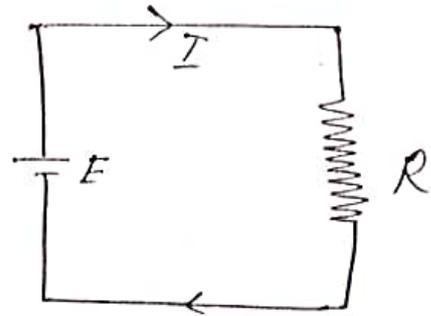
1. The closed path for electric current is called an electric circuit.
