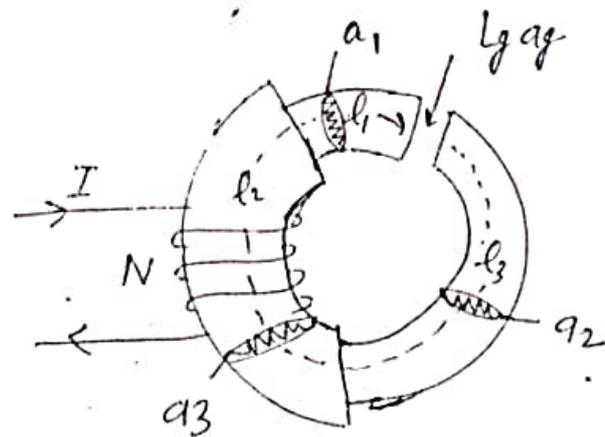
In a Series magnetic circuit, the same flux  $\phi$  flows through each part of the circuit. It can just be compared to a series electric circuit which carries the same current through.
