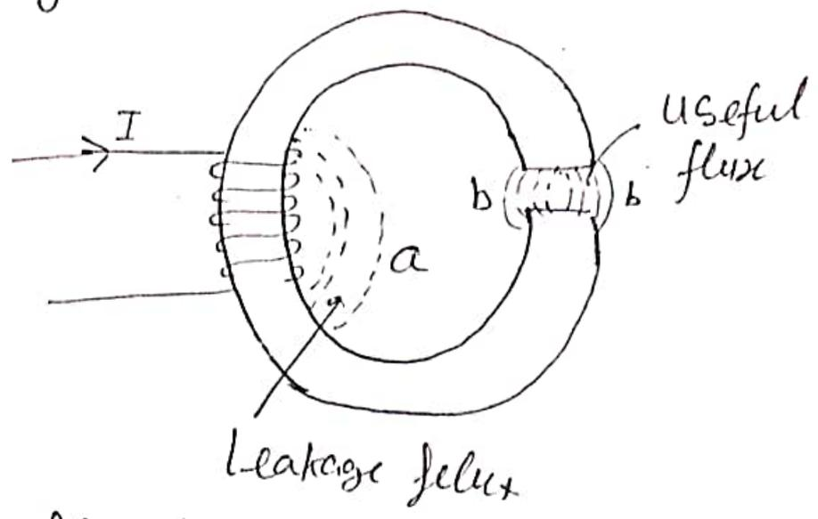
$\Phi_i$  = total flux produced or flux in the iron ring
