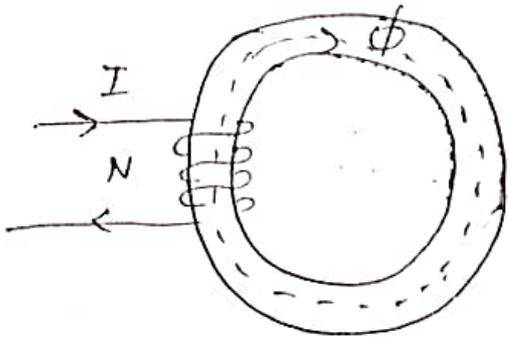
1. The closed path for magnetic flux is called a magnetic circuit
